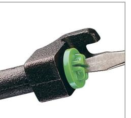
MSP Series plugs feature two concentric raised rings on the underside of the flange to provide a positive seal for metric-threaded parts. Cross-slotted head makes it easy to tighten or remove with a screwdriver.
